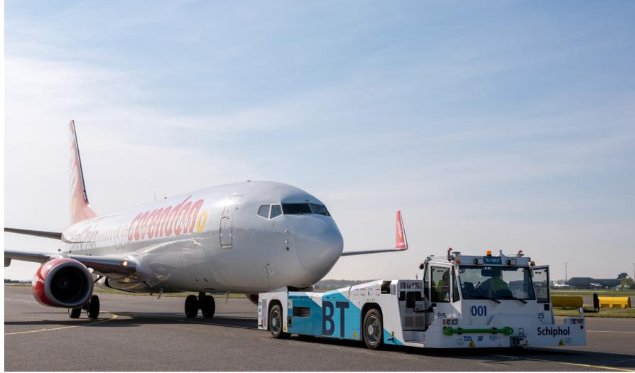
The Taxibot has four-wheel steering, which makes it highly flexible. It can both turn on its axis and drive sideways. The Taxibot connects to the aircraft in such a way that the pilot can steer it with the nose wheel, and the Taxibot's flexibility ensures that it follows the movements of the nose wheel exactly.
